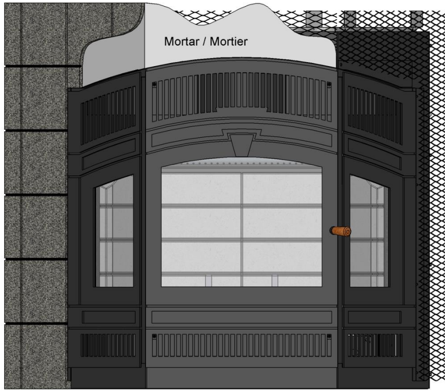
Figure 2 Facing with masonry Devanture de maçonnerie
