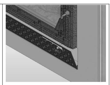
Figure 2 Bottom louver installation
