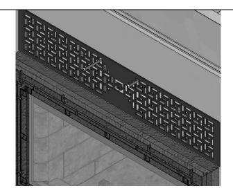
Figure 4 Top louver installation
