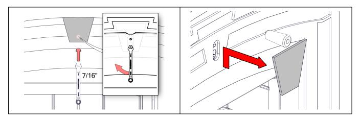
2. Install the bolt support at the top of the louver opening. Center it horizontally in the opening, push up on the inner casing and pull it forward as far as it will go. Install a threaded "U" connector over each hole on the bolt support bracket.
