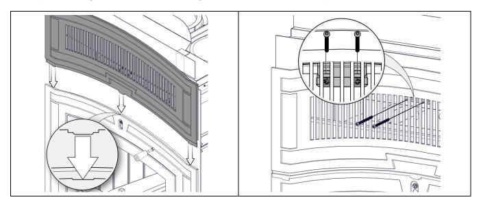
5. Use a <sup>7</sup>/<sub>16</sub>" wrench and screw the nut most of the way on the large keystone. Insert the keystone nut into the decorative facing hole and pull it down in place. Tighten the nut on the back side of the faceplate using the wrench.
